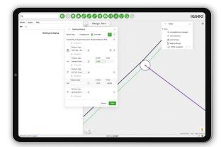
The industry's first staking wizard enables precise digital staking, including GPS locating, wire details, and precise distance and angle designations to accelerate field design
